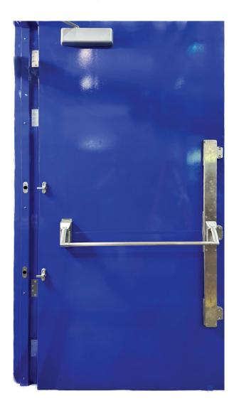
1" throw 304 stainless steel bolts with mechanical deadlock and single motion retraction for egress.
